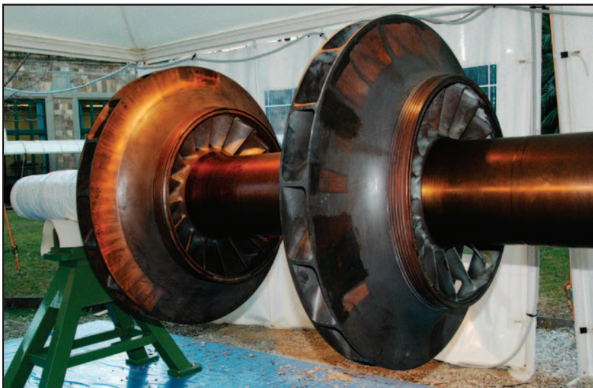
■ Rotor of the MCL 1402 nitrogen compressor for the 7.8 million t/y Qatargas II LNG plant.
