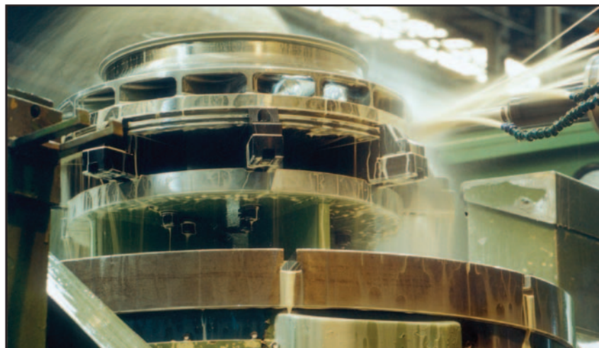
■ Shrouded impeller milled on a 5-axis machine from a single forging.
