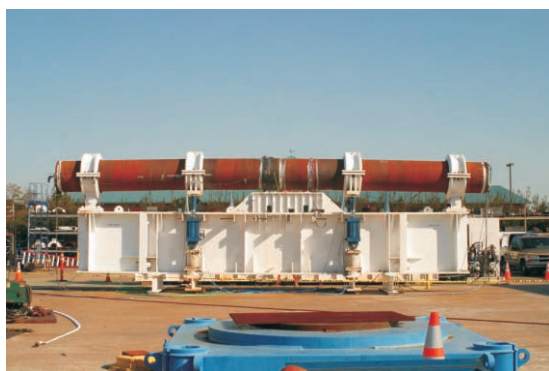
RL-2HCX connector in bend test machine at VetcoGray's R&D facility - Houston (All tests witnessed and verified by DNV)
