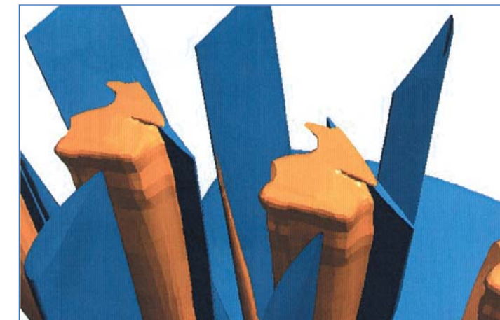
Computational Fluid Dynamics (CFD) model of Mach 1 Iso-surfaces.
