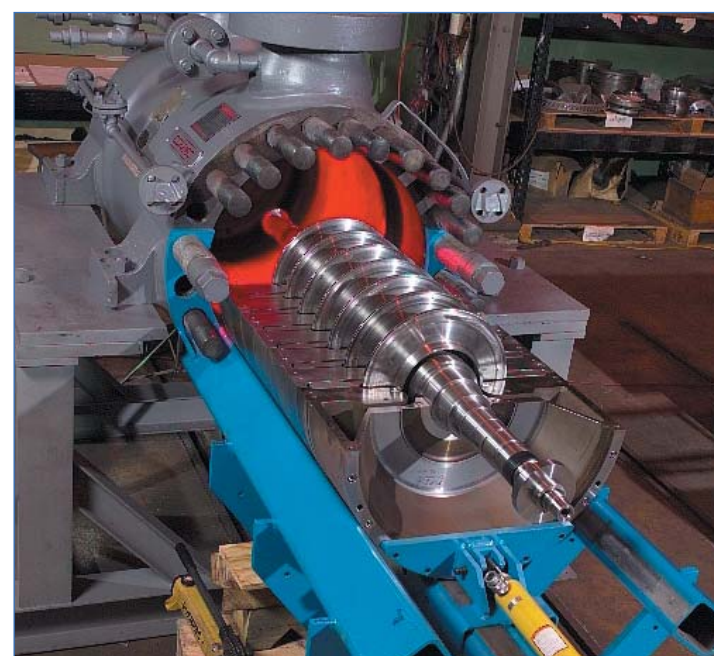
New aerodynamics for H 2 Recycle compressor
