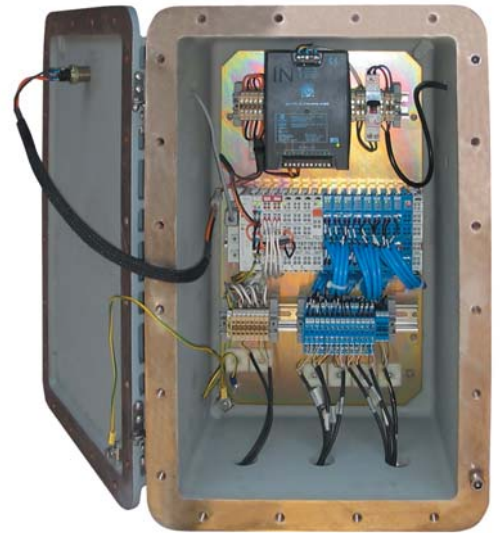
Local data acquisition system
