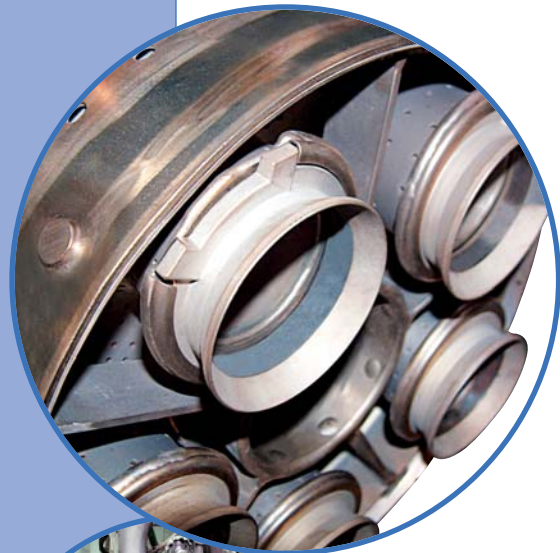
Detail of the DLN liners, redesigned and internally coated
